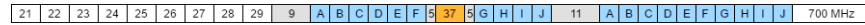
Figure 5: The band plan for the 126 MHz clearing target (the initial clearing target for Stage 1 of the BIA, which subsequently failed). White blocks on the left are TV channels of 6 MHz each and blue are mobile blocks of 5 MHz each. The grey blocks are guard bands. Channel 37 is protected for radio astronomy and wireless medical telemetry use.
